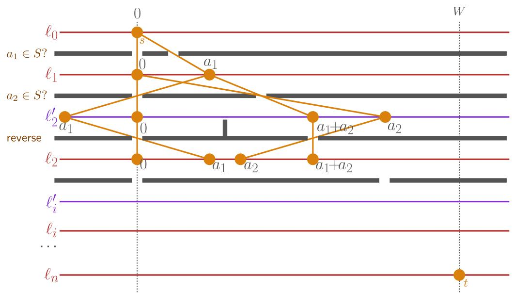
**2-Partition**: n integers  $a_1,...,a_n$  with  $\sum a_i = 2W$ . Is there a subset S that sums to W? Min link path\* with bends on lines,  $\iff$   $\exists$  subset S that sums to W from s to t with 2n-1 links W $a_1 \in S$ ?  $a_1$  $a_2 \in S$ ?  $a_1 + a_2$  $a_2$ reverse  $a_1 + a_2$
